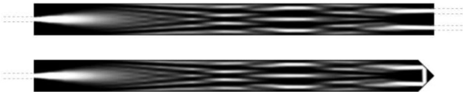
Figure 19.15: Modal propagation simulation of a 1 \times 2 MMI (top) and the corresponding 1-port multi-mode interference reflector (bottom).
