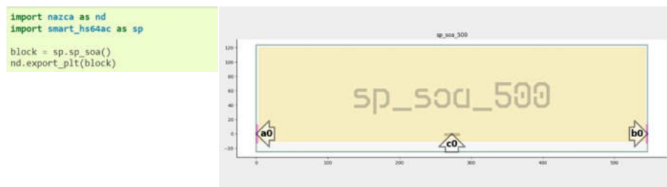
Figure 14.17: Python code snippet to display the image an SOA building block for a 500- \mu\text{m} -long SOA on n-doped substrate. The arrows indicate the connections for the passive waveguide and the electrical connection.
