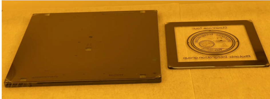
Figure 4.32: Side by side photograph of a 6-inch scanner 4X reticle (left) and a 4-inch 1X contact lithography mask (right) both displayed with chrome pattern side up.
