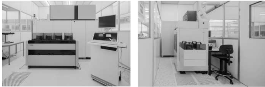
Figure 4.38: ASML tools at Nanolab@TU/e: PAS5500/1100B scanner (left) and PAS2500/40 stepper (right).
