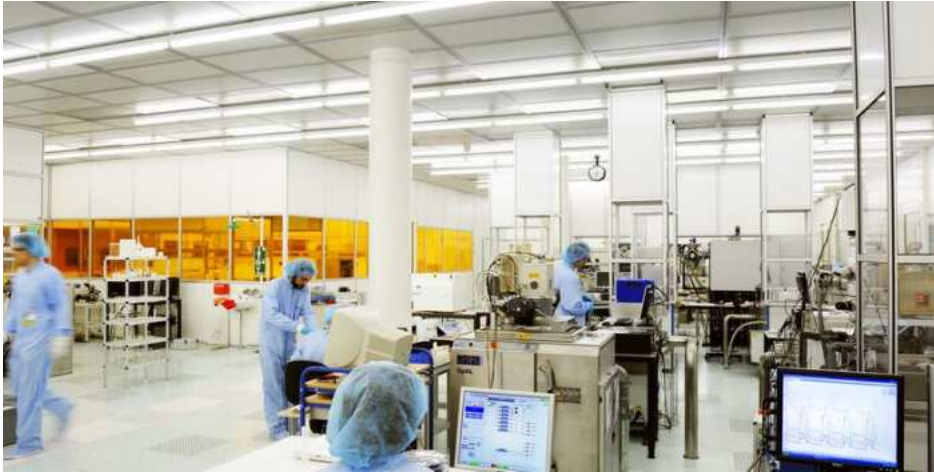
Figure 4.17: View of the TU/e cleanroom with a variety of processing equipment. On the background the (yellow) lithography room.
