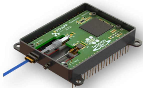
Figure 4: PhotonFirst System-in-a-Package module: integration of electronics and optics.
