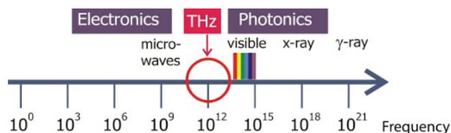
Figure 1: Electromagnetic spectrum with the THz radiation located between the visible light domain and the microwave domain, from [3].
