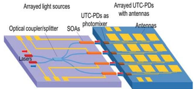
Figure 3 Schematic view of arrayed light sources and arrayed UTC-PDs<sup>8</sup>.
