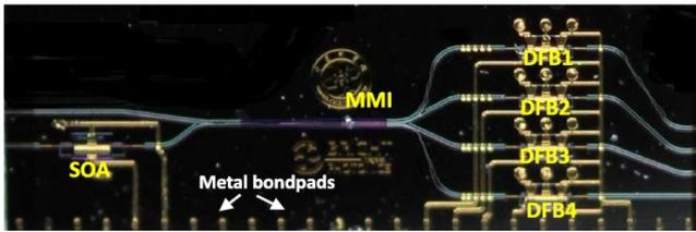
Figure 2 (a) Layout and (b) microscope view of the monolithically integrated THz PIC optical heterodyne<sup>2</sup>.
