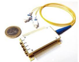
Figure 2: InP monolithic integrated photonic microwave filter. From [7].
