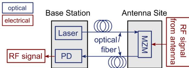
Figure 1: Scheme of a remote ROF receiver antenna for remote receiving.
