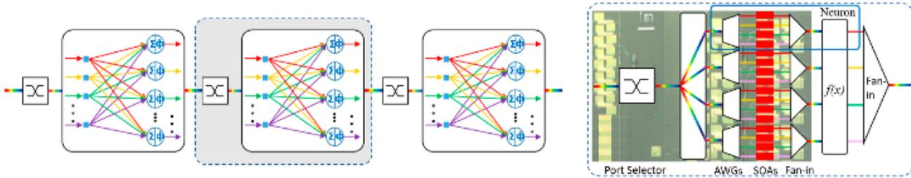
Figure 2 Scheme of a three-layer photonic deep neural network. The included port selector may be used to be used to select the desired input source. One full layer of neurons by exploiting onewavelength divisionmultiplexing (WDM) input, with a shaded photonic integrated circuit micrography at the back, to underline that part of the circuitry that is realized on chip. From [4].
