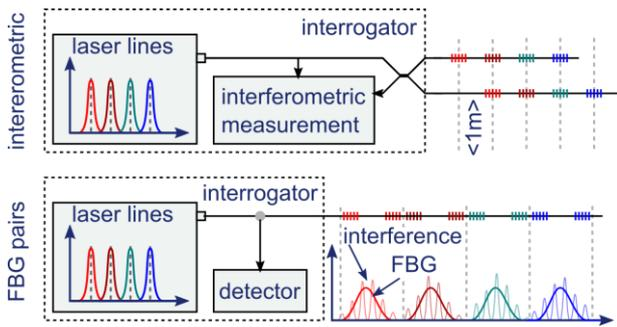
Figure 2 Two common fiber sensing concepts using wavelength multiplexing. Top: interferometric fiber sensing. Bottom: interferometric sensing using FBG pairs.
