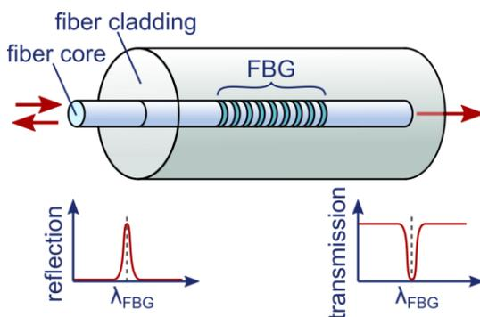
Figure 1: Schematic view of a FBG, with the refractive index modulation indicated on the fiber core and illustrative transmission and reflection spectra.
