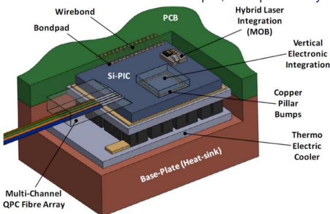
Figure 2: Schematic of a packaged silicon PIC with hybridly-integrated InP laser, based on a micro-optic bench. Image courtesy of Tyndall [1].
