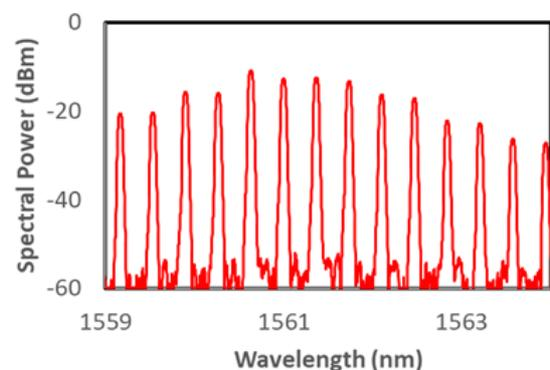
Figure 1: Output of an InP-based mode-locked laser diode, fabricated in the SMART Photonics platform. The comb of equally-spaced optical frequencies can be used as efficient WDM sources for a silicon PIC. Image courtesy of Aarhus University.
