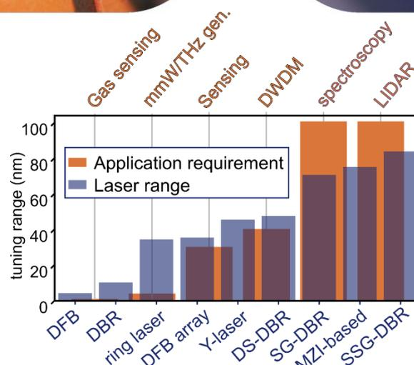
Figure 1: Comparing application required wavelength coverage and tunability of InP laser technologies.
