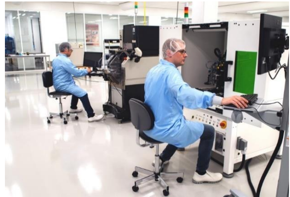
Figure: Packaging equipment (Technobis): fully automated wire bonder and die bonder in use 2,3 .
