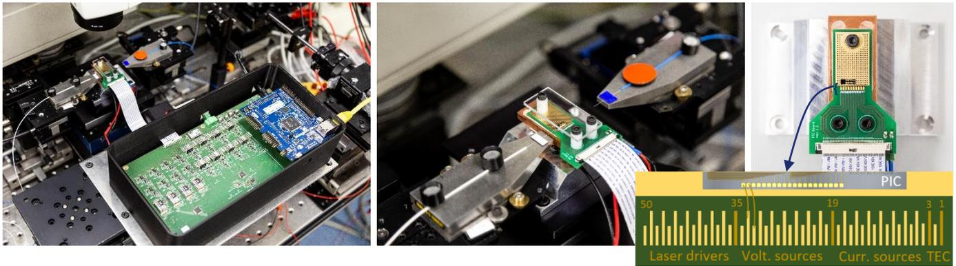
Figure 2: PICConnect mainboard with microcontroller board and PIC Board integrated in a measurement setup (left). PIC Board mounted and assembled (centre), with a close-up of the PIC Board on the top right and the pinout of the PIC Board bond pads on the bottom right.
