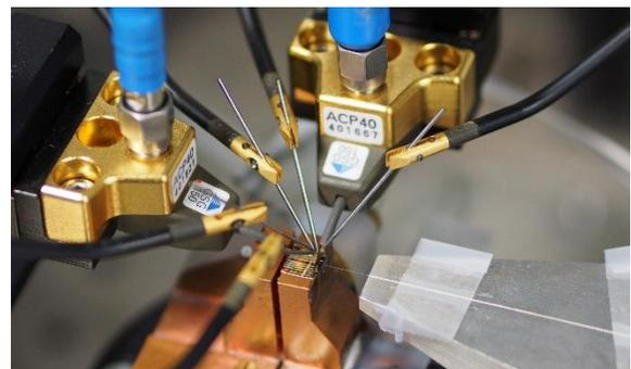
Figure 1: Probing of a PIC with RF and DC probes (image courtesy of Weiming Yao).
