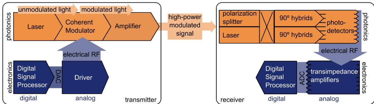
Figure 2: Photonic and electronic components of modern coherent transceivers.
