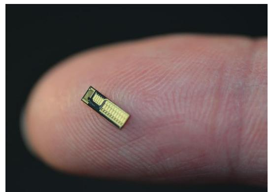
*Figure 1: EFFECT Photonics optical ‘System-on-Chip’ – including actives and passives on a single chip, illustrating the potential for form factor reduction.*
