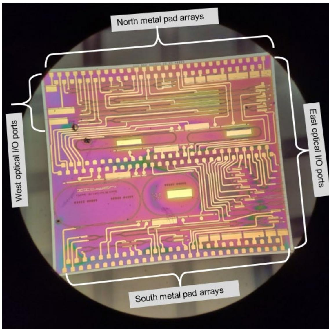
Figure 1. Typical PIC under a microscope.
