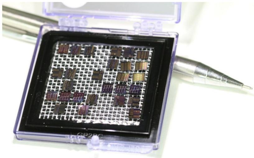
Figure 2. PIC chips in a gel-pak box.
